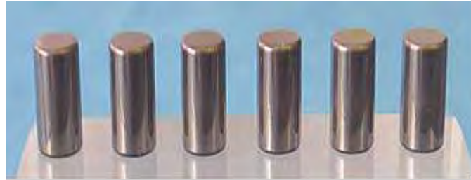
Fig. 4: Silicon carbide based roller bearings manufactured by extrusion of Si- and SiC-loaded polysiloxane polymer.
